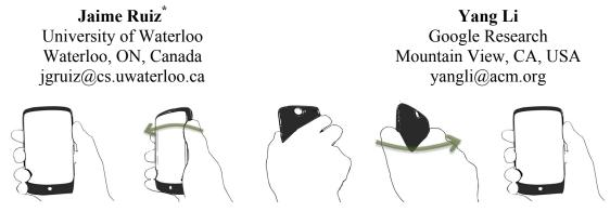
Figure 1: An illustration of the DoubleFlip gesture. In this figure, the user holds the phone right-handed. He rotates the phone along its long side so that the phone screen is away and then back.
