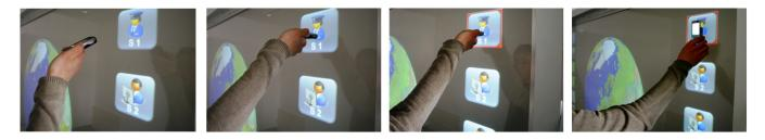
Figure 2: Interaction scheme to authenticate with a specific user role on an FTIR multi-touch surface: (i) The user touches the wall with the phone. (ii) The mobile phone flash light sends a light flash (or a camera flash) to indicate the region the user wants to interact with and at the same time initializes the authentication process. (iii+iv) The user can interact in his/her assigned role with the wall and do critical actions.
