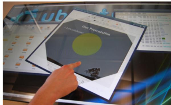
**Figure 8. Rotation and translation in the Manipulate plugin using one finger.**
